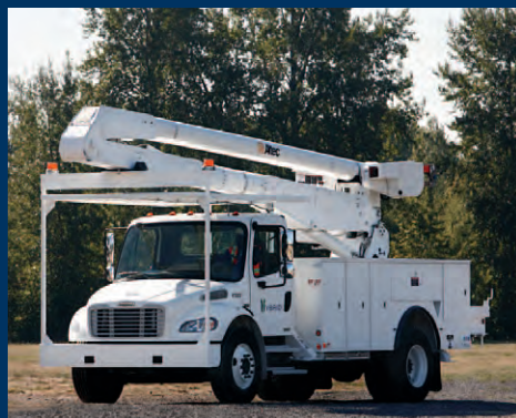
Freightliner Business Class M2 106 Hybrid With parallel-electric hybrid system
