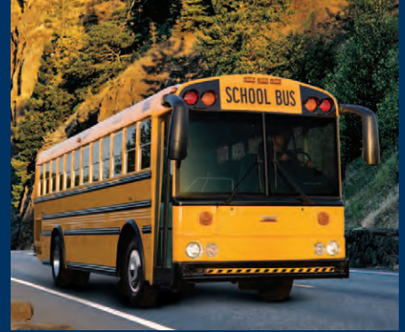
Thomas Built Saf-T-Liner HDX With natural gas drive system
