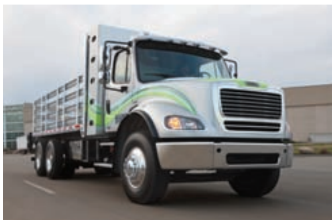
Freightliner Business Class M2 112 Compressed Natural Gas Truck
