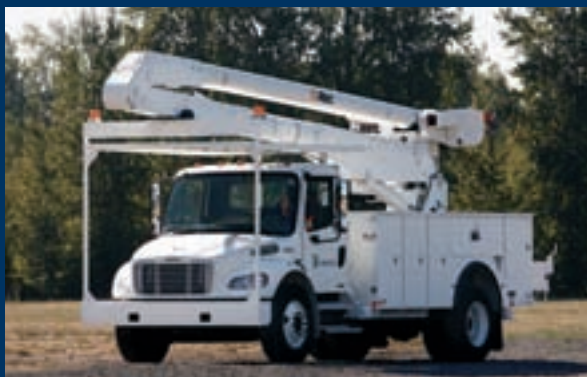
Freightliner Business Class M2 106 Hybrid With parallel-electric hybrid system
