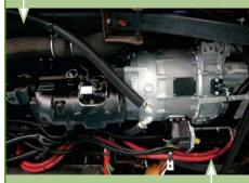
ELECTRIC DRIVE: Electric motor, output 44kW, generator output 44kW
