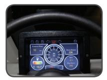
DISPLAY PANEL Informative and concise, our display panel shows standard information including vehicle speed, odometer, shifter position, turn signals, emergency flasher indicators, and parking brake indicator. The panel clearly shows estimated range, as well as, the battery charge status. The amps indicator will help drivers attain maximum efficiency.
