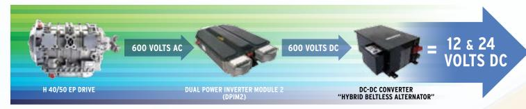
Allison has taken the next major technology step with the introduction of DC to DC converter capabilities. A solid-state DC to DC converter eliminates the traditional alternator to provide greater reliability while lowering operational costs and maintenance issues. The converter will not use the ESS2 for any stored energy, thereby maintaining our unequalled hybrid battery life.
