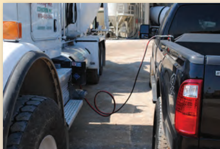
Ward Alternative Energy Service Truck providing Off-Load Fueling to Loveland Ready Mix Truck
