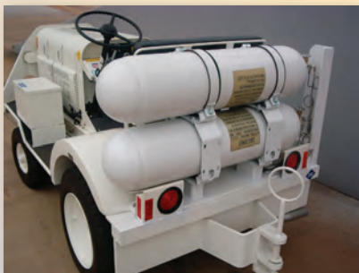
FuelTek CNG Conversion for Airport Baggage Tractor
