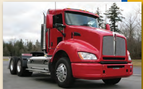
Kenworth Class 8 CNG Tractor with 80 Diesel Gallons Equivalent Fuel Storage
