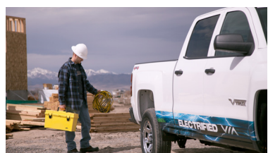
The onboard generator provides a work site with 14.4 kW of exportable power
