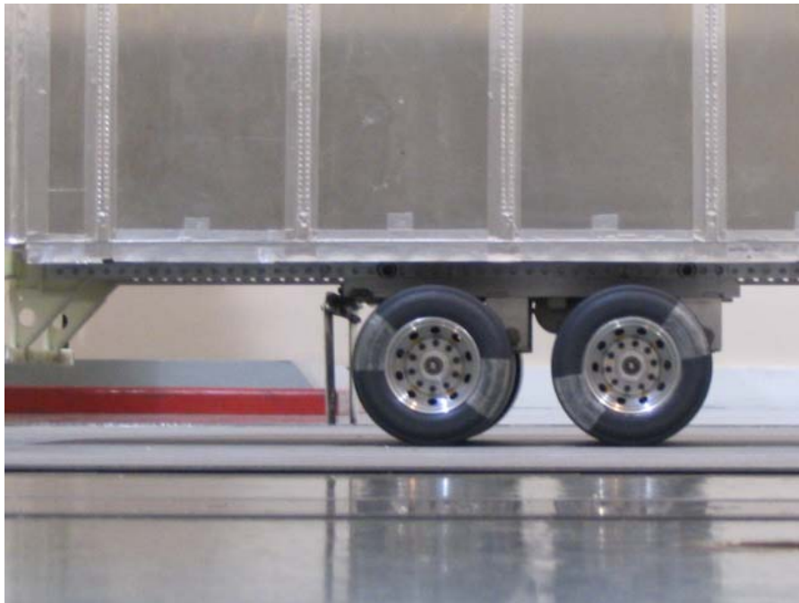
Trailer Boggy positions is 40' from the center line of rear axle to the king pin
