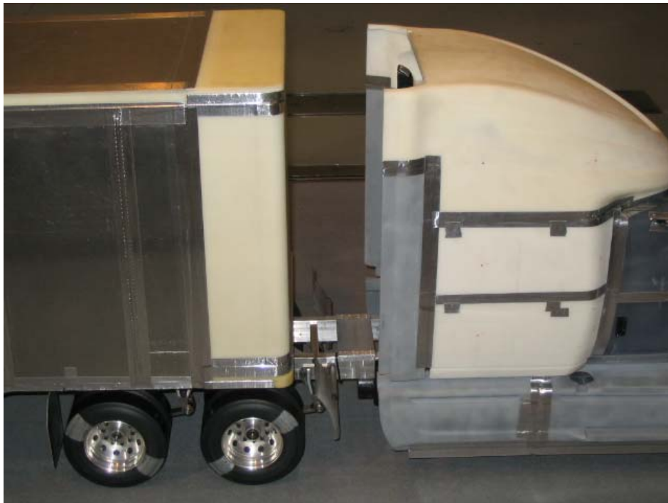
Tractor/Trailer Starting Configuration - Truck to trailer Gap of 45" with a 36" trailer king pin position
