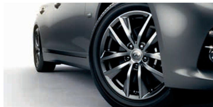
17 INCH, 5 DOUBLE-SPOKE ALUMINIUM-ALLOY WHEELS WITH RUN-FLAT TYRES
