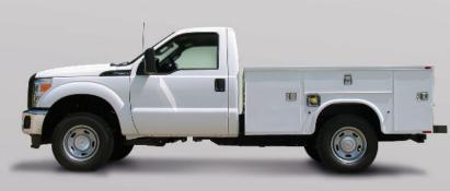
Low Profile Bodies offer greater visibility from the cab while only sacrificing 4" of body height compared to a standard service body.
