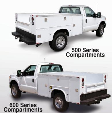
The 500 Series Service Bodies feature a horizontal compartment that stretches from the first vertical compartment to the end of the body with a small rear lower compartment. 500 Series compartment configurations are available for most Service Body models.
