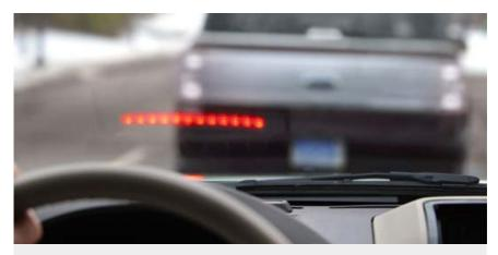
Visual warnings from Ford's Collision Warning with Brake Support technology
