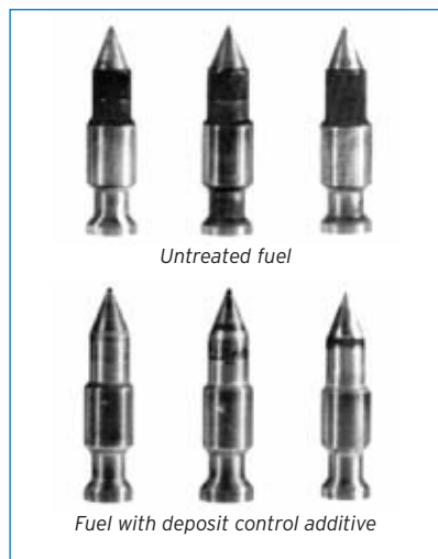
Figure 7.2 Typical Deposit Levels on a Fuel Injector Plunger Susceptible to Deposit Formation
