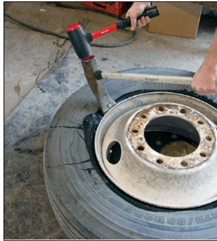
2 Or a duck bill hammer as a wedge, with a rubber mallet.
