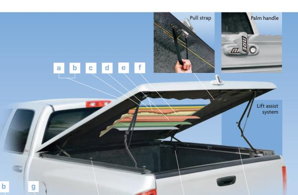
The weight of the cover rests on the height adjusters to protect your truck from unnecessary
