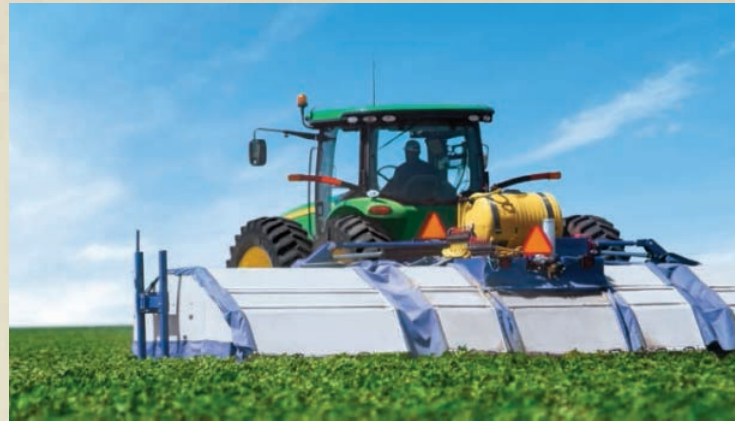
Using computer vision and artificial intelligence, Blue RiverTechnology's smart machines can detect, identify, and make management decisions about individual plants in the field.
