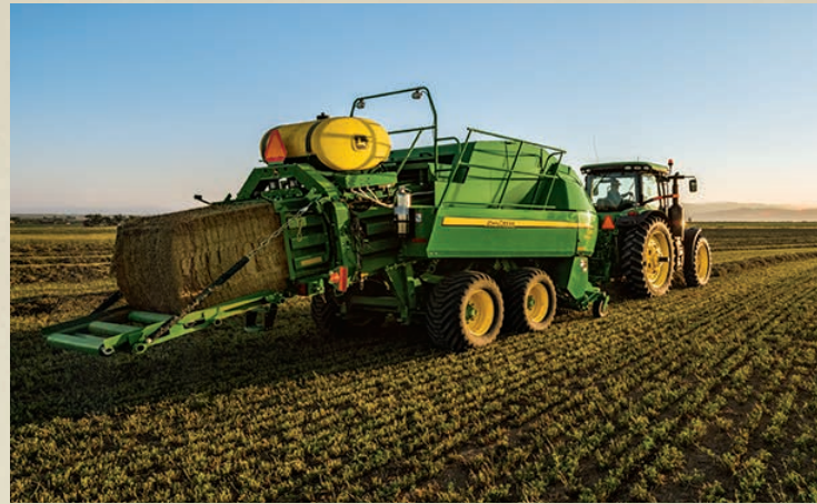
Updated large square balers deliver technology improvements, including an integrated moisture sensor, a bale weighing system, and the ability to clear the feed system from the tractor cab.
